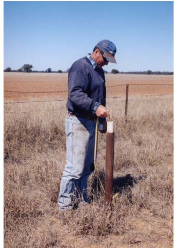
Above: Jeff Betts measures the depth of the water table by lowering a length of tape with a plopper, into the piezometer.
