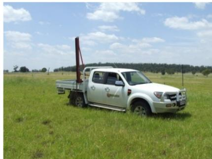
Figure 2: Hydraulic ram on utility for deep coring
