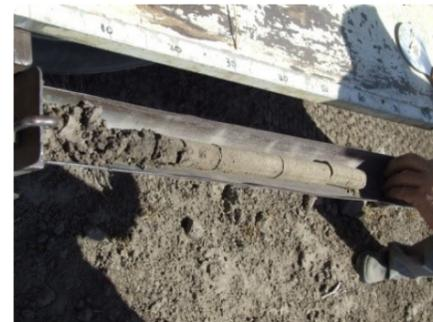
Figure 3: Deep soil core laid out in tube and cut to depth sections
