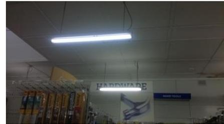
Changing the lights to 18W LEDs would halve the electricity consumption in the store and therefore save the owner thousands of dollars each year. Of course, the business would need to invest in new LED bulbs, but with the considerable savings offered by LEDs, the payback period on the initial outlay would be less than two years.
